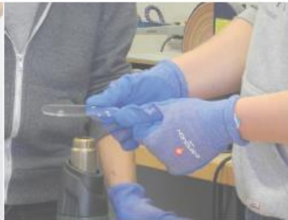
PMMA warm verformen
